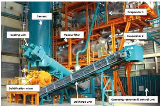
Batch vacuum mixer with solidification unit for treated material. Source: ECON Industries GmbH
