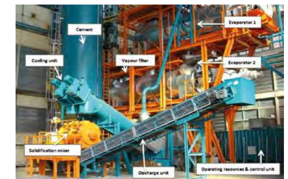
Batch vacuum mixer with solidification unit for treated material. Source: ECON Industries GmbH
