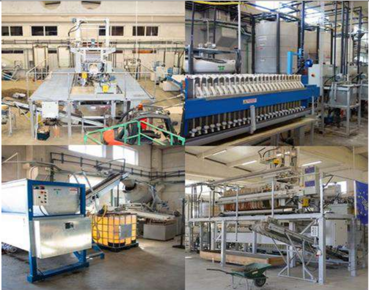
Figure 12: Stationary ReSoil® facility with capacity of 6 t/day constructed under LIFE+ programme .
