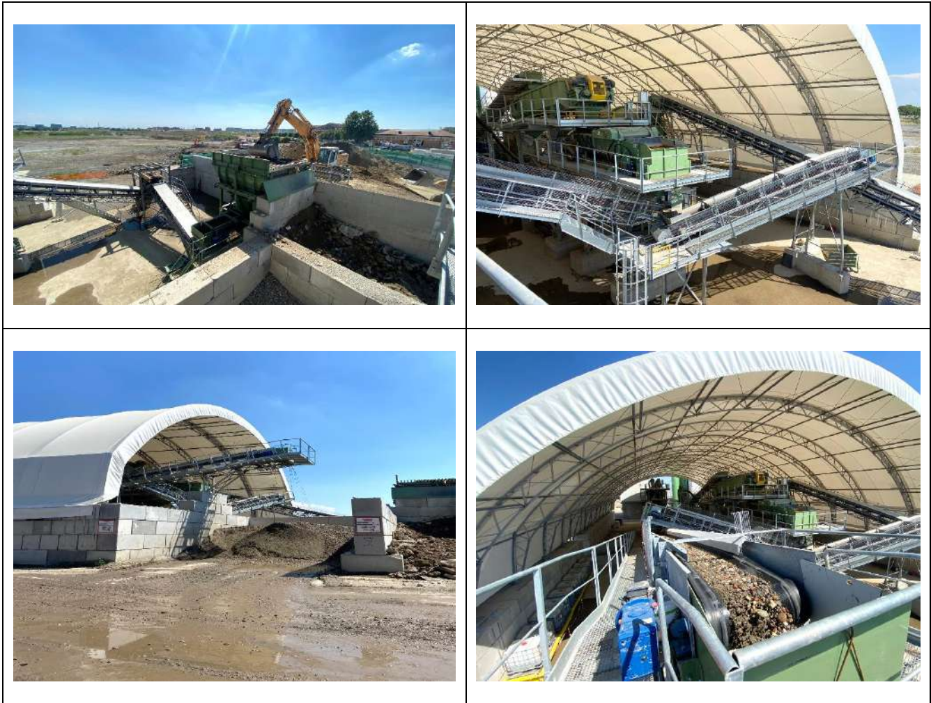
Figure 2.2- Soil washing process (photos by Massimiliano Confalonieri)
