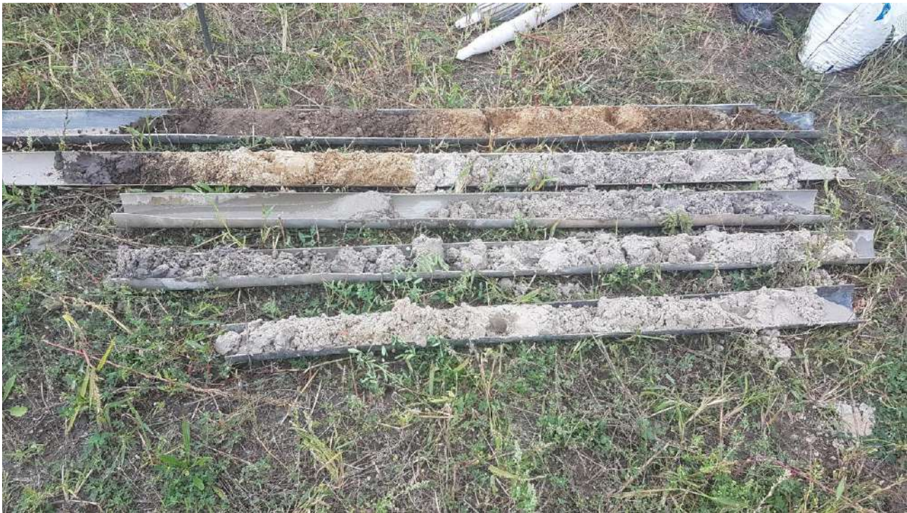
Drill core borehole (sonic drill)
