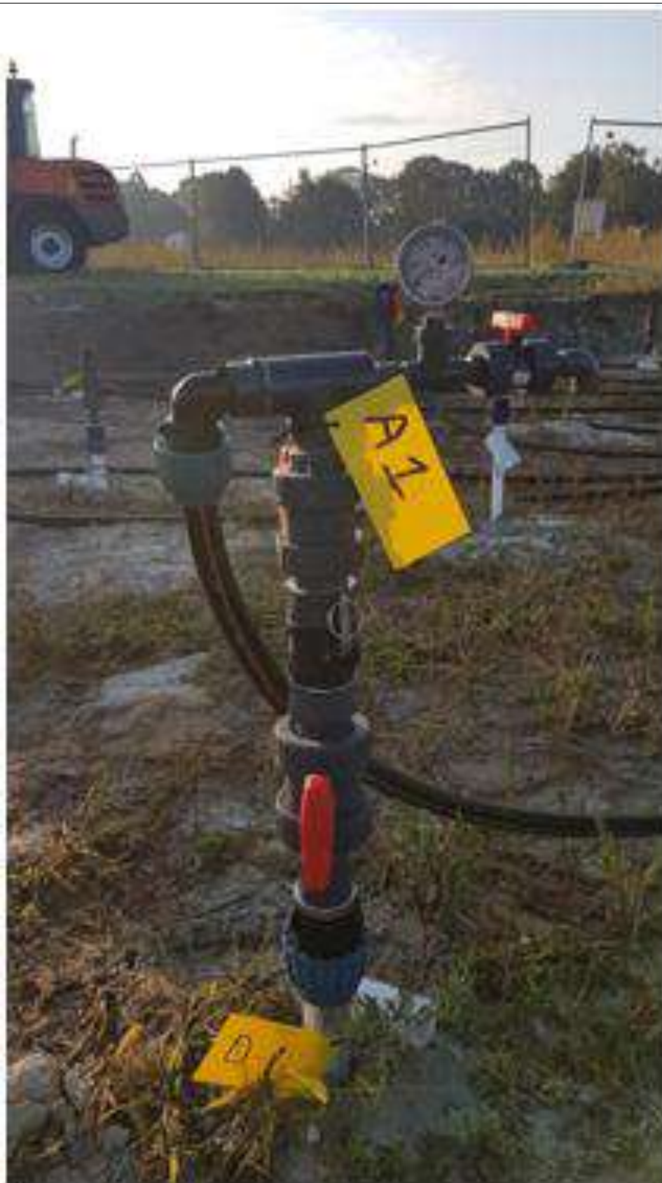
Detail injection well manifold
