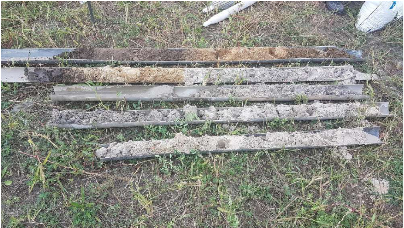
Drill core borehole (sonic drill)
