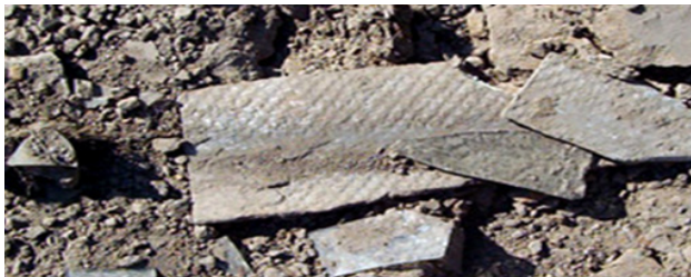
Asbestos cement fragments in soil | AECOM
