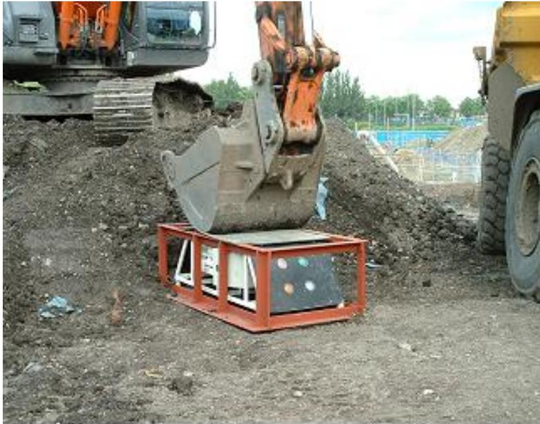
**Figure 3 Photograph showing the GEM system in operation with the loaded excavator bucket placed over the detector, thereby initiating a proximity switch the start the analysis.**
