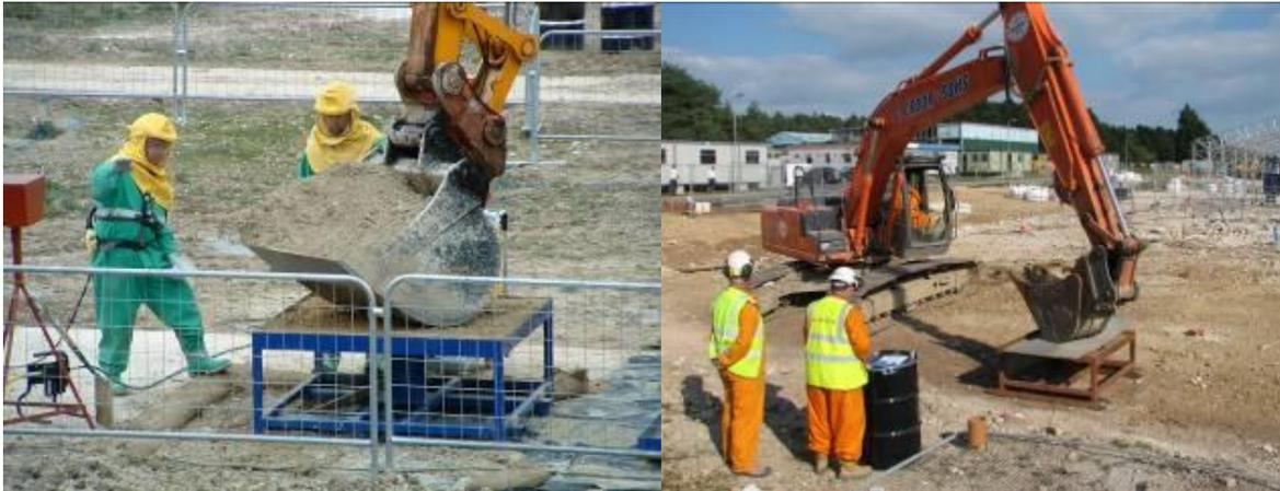
**Figure 2 Photograph showing the operation of the gross gamma system with the detector placed in the centre of a shielded frame over which the bucket was placed.**
