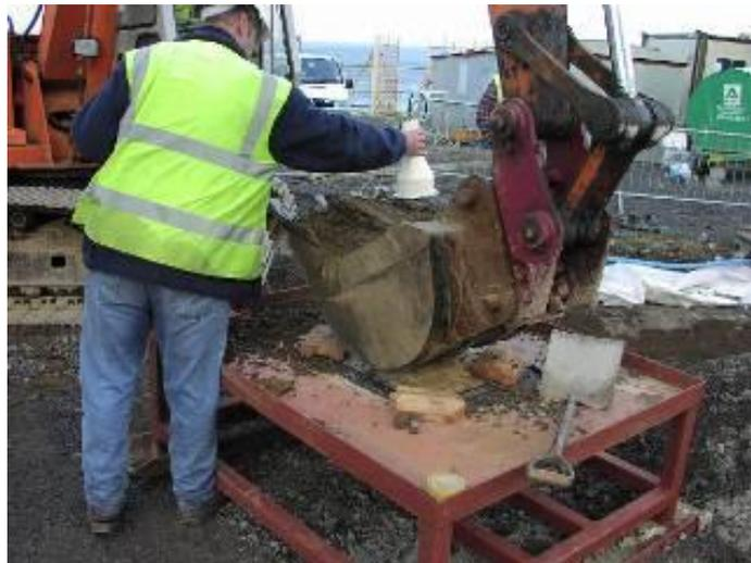
**Figure 1 Photograph showing an excavator bucket load of soil being monitored using a hand-held instrument.**
